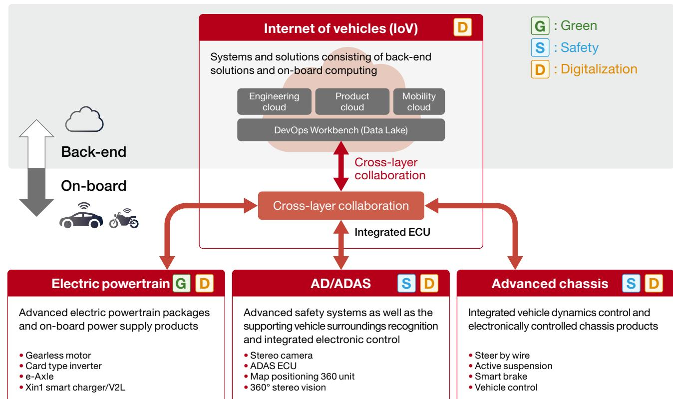
AD: Autonomous driving / ADAS: Advanced Driver / Assistance systems / DGM: Detailed Geometry Map / e-Axle: Electric axle
