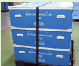
Using hook-and-loop fastener-type cargo restraint bands
